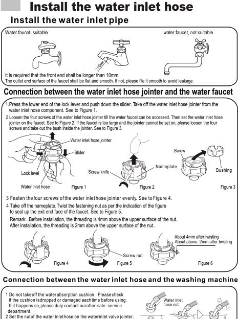
3 Fasten the nut. Swing it gently to confirm if it's fastened well. Water inlet valvejointer
